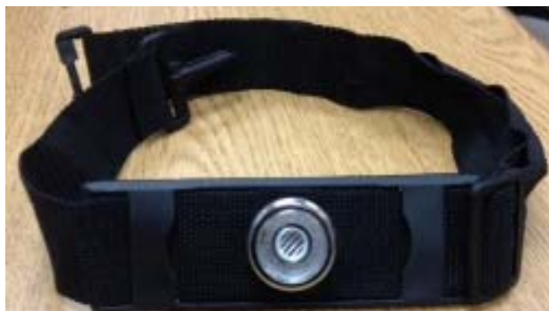
Figure 2. The microphone in the stethoscope and its neck band.
