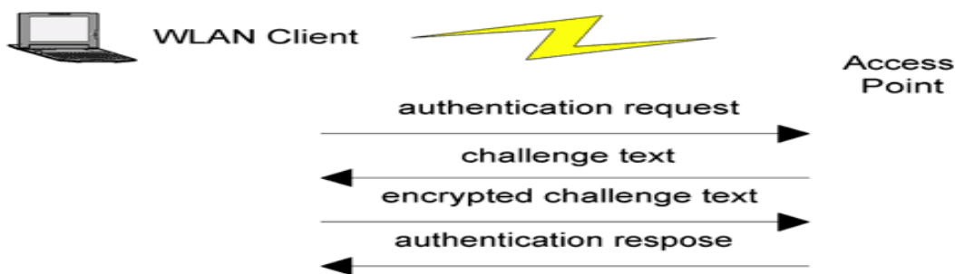
FIGURE 3 WEP SHARED KEY AUTHENTICATION PROCEDURE [21]
